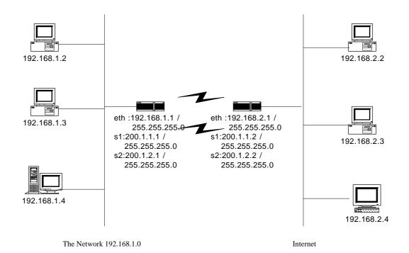
When A & B are communicating, you can activate the serial line redundancy to deal
