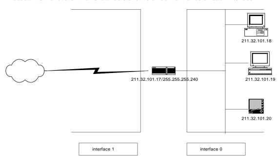
It represents the information of traffic which is for the interior ip when enable ipaccount to the interface which linked with the interior.
