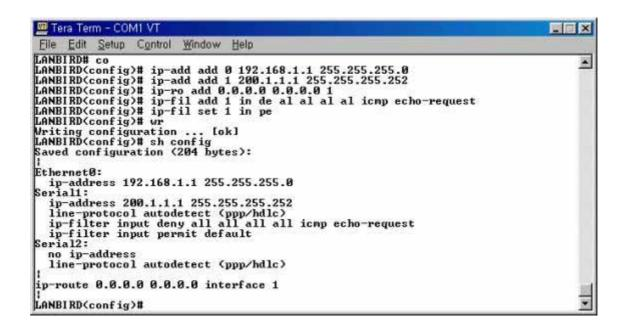
To block telnet connection from the network 100.1.1.0 to the network 192.168.1.0, you need to block the telnet port which comes from the network 100.1.1.0 or block syn packet which is willing to do telnet connection. After that, permit other packets.
