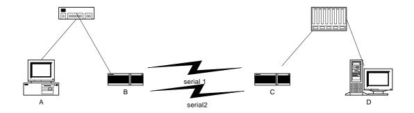
When host A is connecting with the remote server D, you can activate the load balancing through serial1 and serial2 between B and C. Host can be served by server through load balancing.
