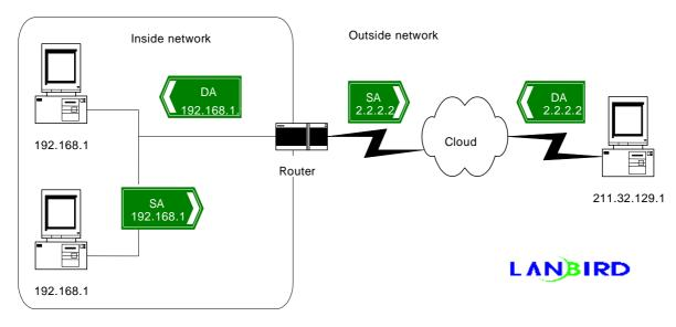
The following procedure shows the example of using Internet through changing the source address of the host with the a inside private address by a router in the above figure.
