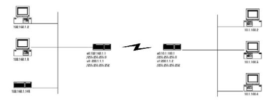
As the figure above, from the router 192.168.1.1 to the network 10.1.100.0, routing goes through the serial interface. If the default path is 192.168.1.143, the loop remains within TTL(Time To Alive) when the serial interface is down.
