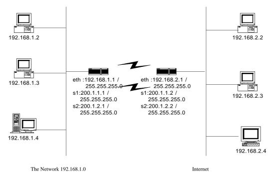
When A and B are communicating, you can use serial1 and serial2 to break up the traffic.
