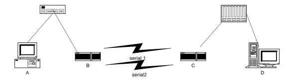
In case that the host A connected with the server D and the serial 1between B&C is down, consequently, the host will be served by server D continuously via serial2.
